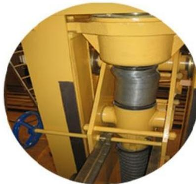
3. Jacks are equipped with infrared sensors which make an emergency stop of jacks at getting of foreign subjects or the personnel in "dangerous zones", at rise or lowering.
